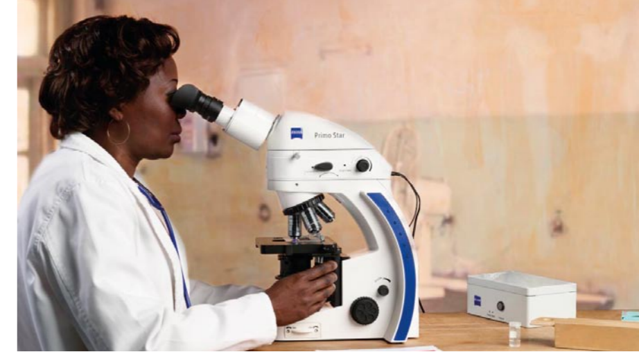
The LED-based fluorescence microscope Primo Star iLED simplifies the microscopic analysis of pathogens
